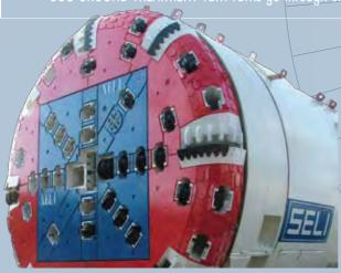
DSU Ground Treatment TBM has been studied and manufactured for the construction of the Tunnel of Abdalajis East for the High speed Railway Project Cordoba – Malaga ( Spain ).
