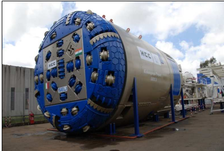
Figure 4. Kishanganga TBM DSU
